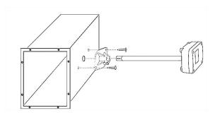
When installing the product, please keep the direction of the arrow on the probe and the direction of the wind.
